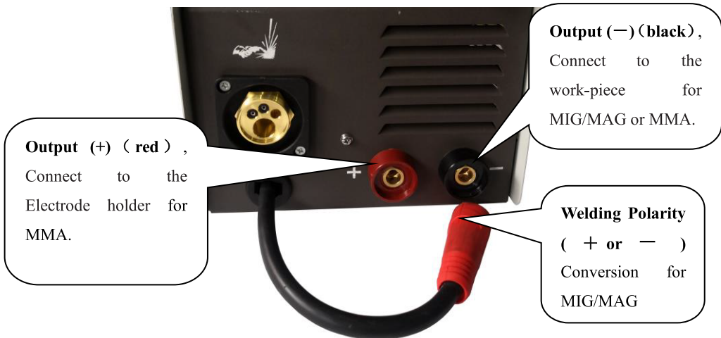
Fig.3: The front panel of the welding power source
