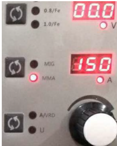
Fig. 9: MMA welding method without VRD ('A/VRD' LED is not lighted)
