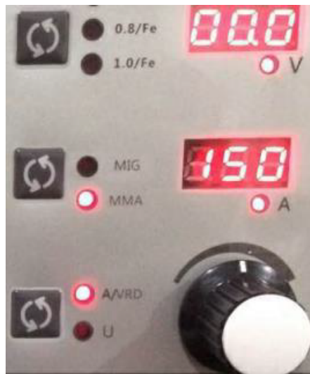
Fig. 10: MMA welding method with VRD ('A/VRD' LED is lighted)
