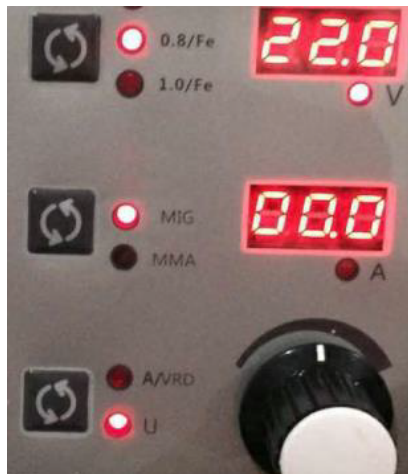
Fig. 11: Under 'U' LED is lighted and flashing, Set welding voltage (V) for MIG/MAG welding method For example, Operating method for MIG/MAG(CO 2 ) welding
